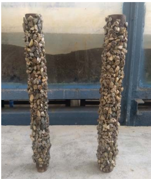
( Figure 2- piers with roughness 7.5 mm)
